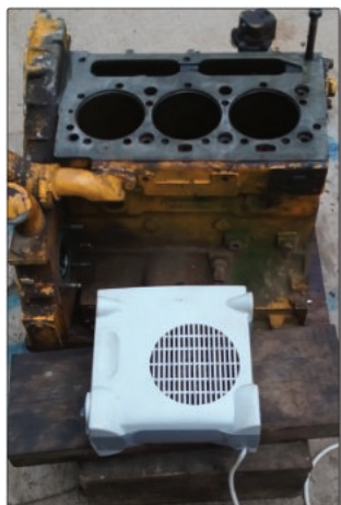
Heating the engine block to receive liners
