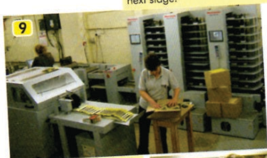
9 General view of the book-let finishing machine. The printed sheets go into the bins behind the operator. They are automatically collated together, folded, stitched and trimmed.
