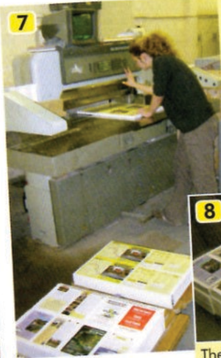
7 After allowing time for the ink to dry, the printed sheets are cut ready for making into books.
