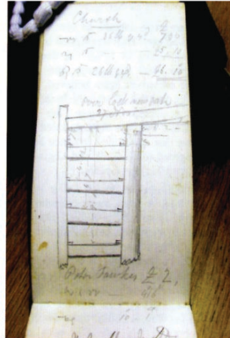
Above: Stephen Ballard's notebook sketch of a gate for Over Lock.
