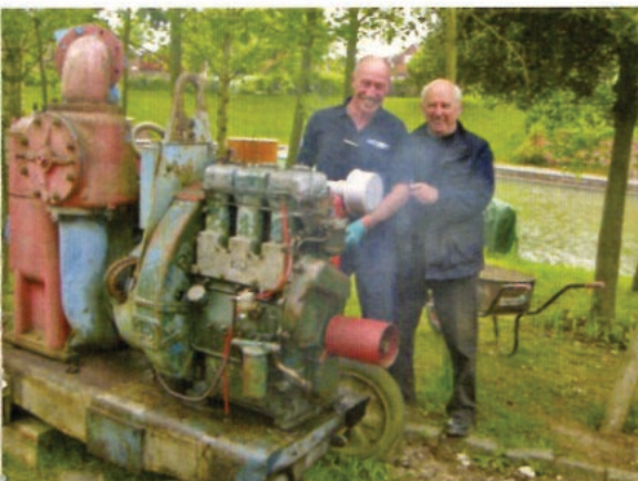
Above: Working on the refurbishment of the old Sykes pump in the compound at Over.
