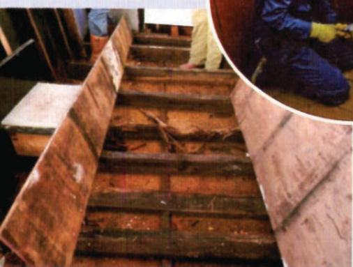
The rotting floor boards on Mister Maysey are all being ripped out and replaced as part of the cabin refurbishment.
