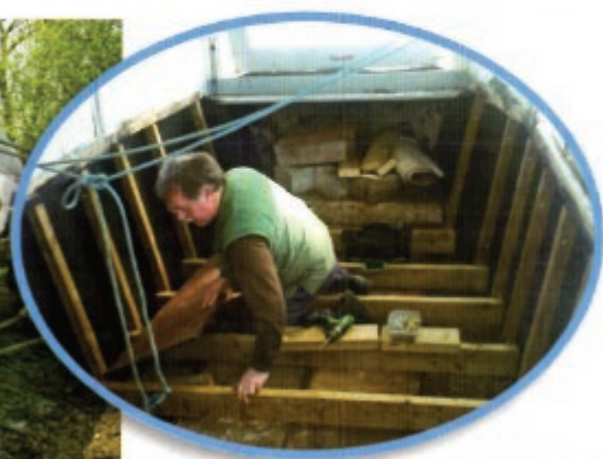
Whilst outside the hull is prepared and painted, new floor joists are fitted within the hull of Mister Maysey.
