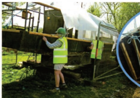
Whilst outside the hull is prepared and painted, new floor joists are fitted within the hull of Mister Maysey.
