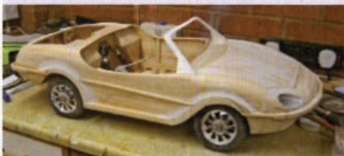
Below: Marine plywood sheeting underside and lime planks were used for the curved wings and bonnet.
