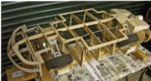
Above: Bob's Amphicar has plywood frames.
