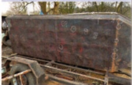
Below: Repair site on the hull of the reed cutting boat.
