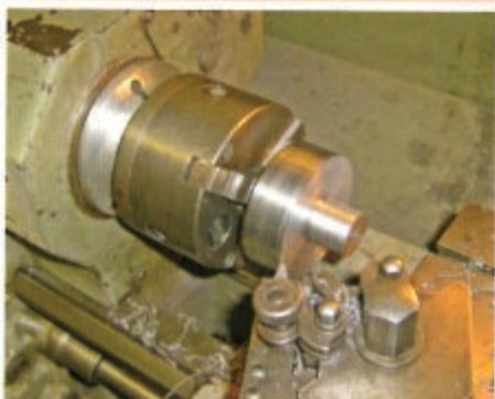
Turning the roller profile.
