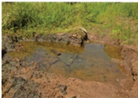
Trial excavation in the exposed canal bed investigating the puddle clay.
