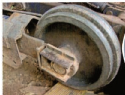
The failed excavator track idler wheel during removal ...
