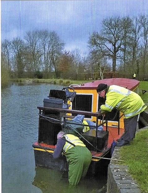
Mike, Dave and Graham remove the rudder to enable access to Mister Maysey's engine.
