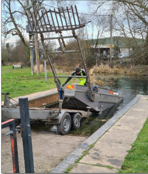
Launching the picking up boat. They have an electric winch within the trailer that controls the launch.
