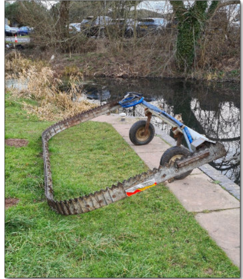
The cutting head ready to load on the cutting boat.
