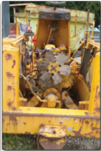
The engine re-assembled, hoisted up and back into place awaiting re-connection of fuel system etc
