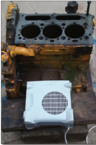
Heating the engine block to receive liners
