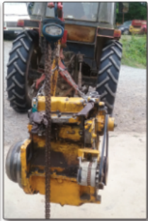
The engine re-assembled, hoisted up and back into place awaiting re-connection of fuel system etc
