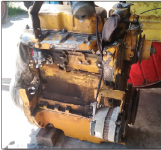
The engine re-assembled, hoisted up and back into place awaiting re-connection of fuel system etc
