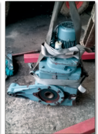
The biodisc unit with distressed 80mm driveshaft and drive train removed and the drive train ready for refitting.
