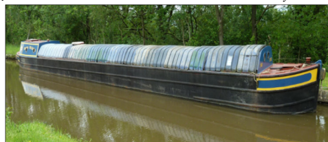
Sister River Class narrow butty boat “Yeo” in original condition with its distinctive glass fibre hatch covers
